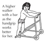
These walkers can be made out of welded or bolted metal tubing.
